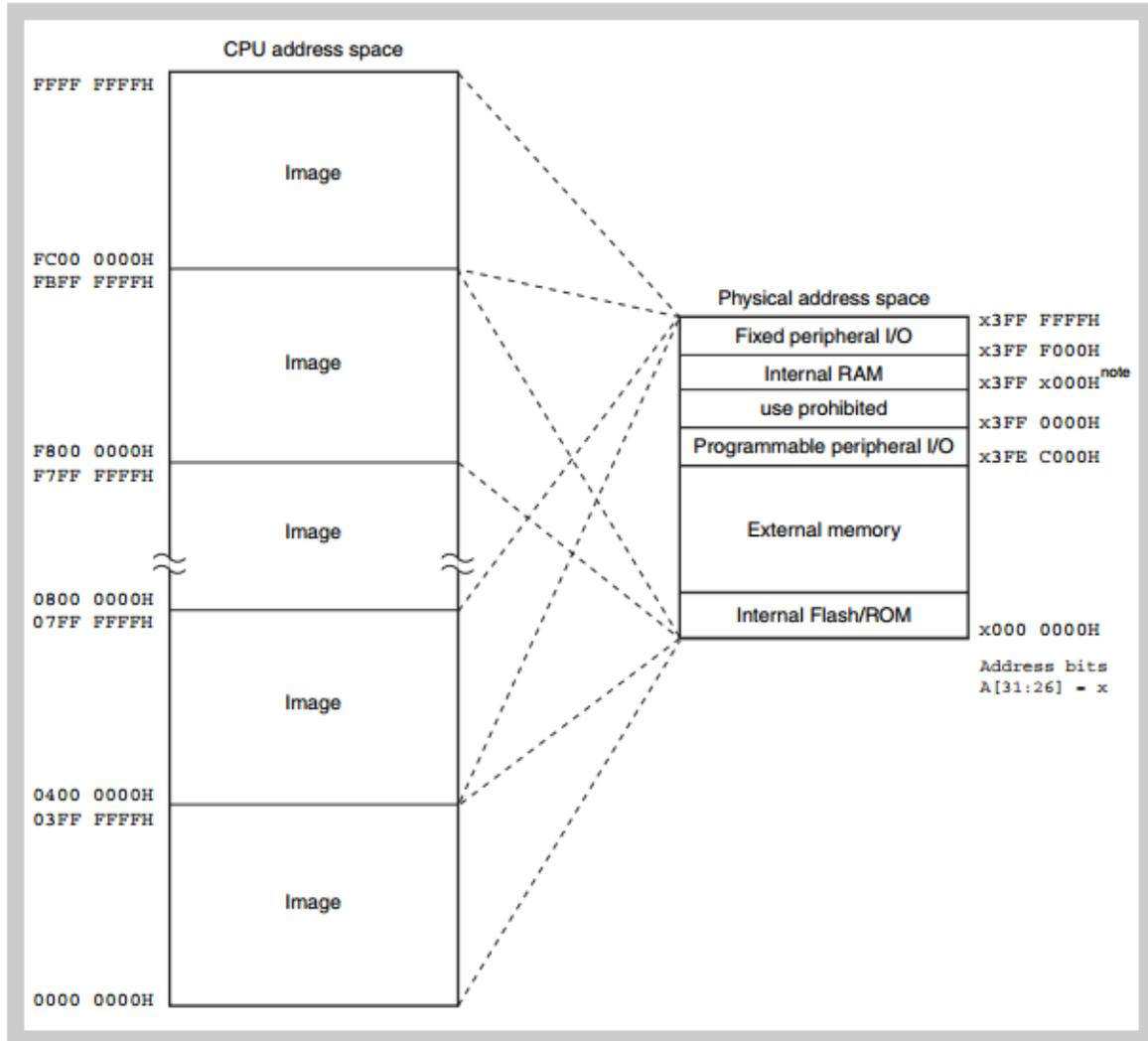
Figure 3-3 Images in the CPU address space
