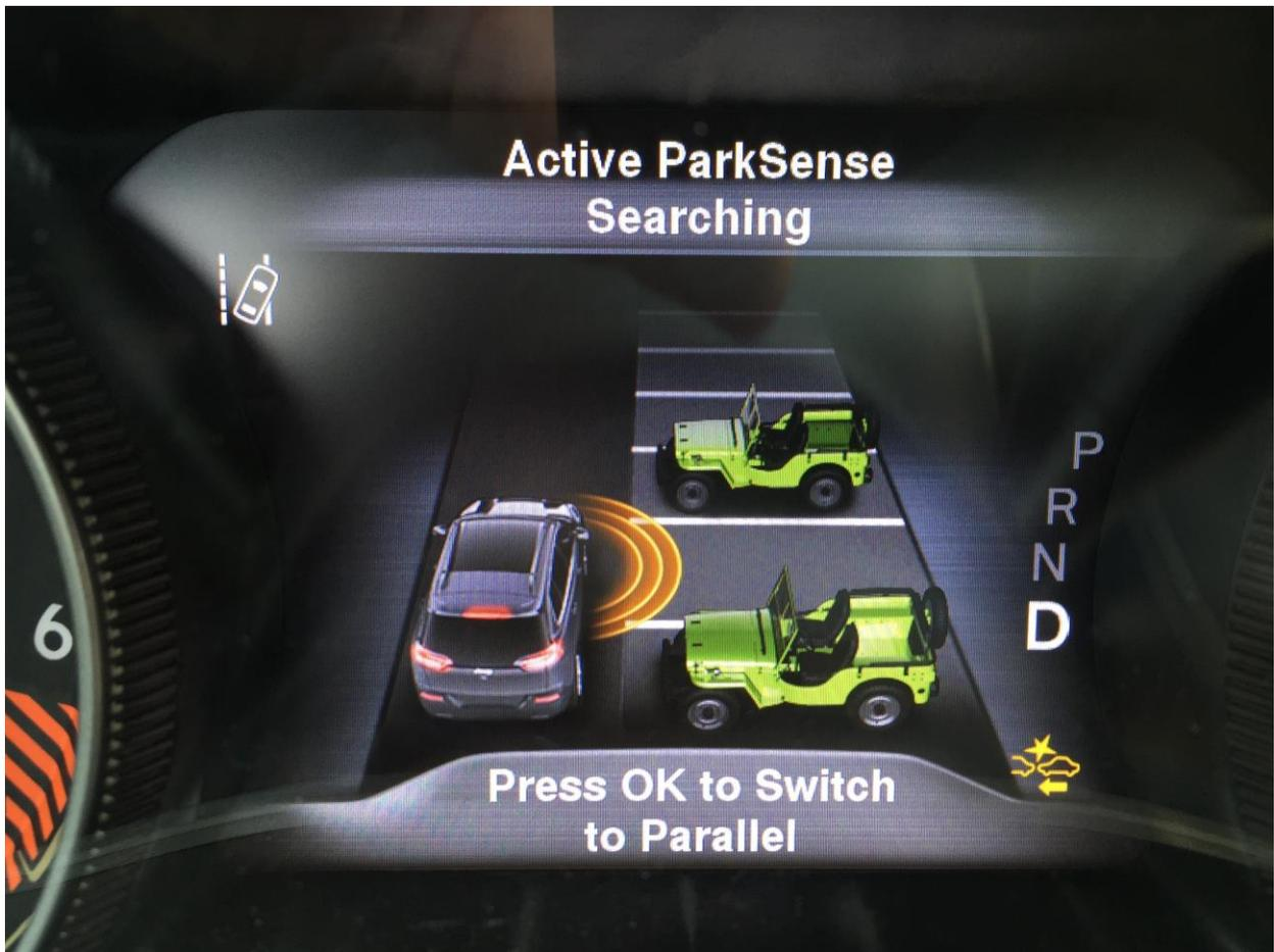
*Figure 5: Display while using PAM system*
