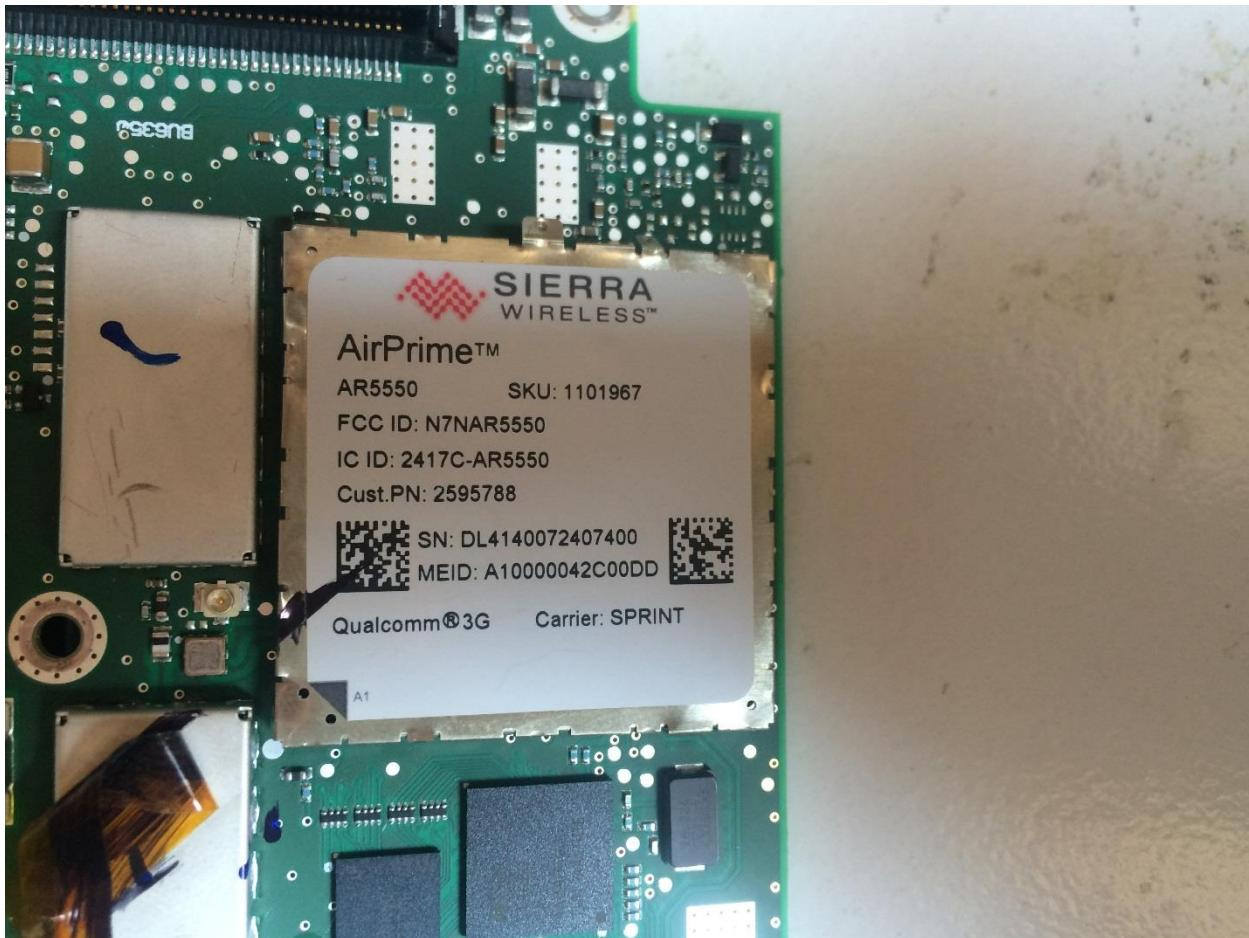
Figure 16: Sierra Wireless AirPrime AR5550 from a Harman Uconnect system
