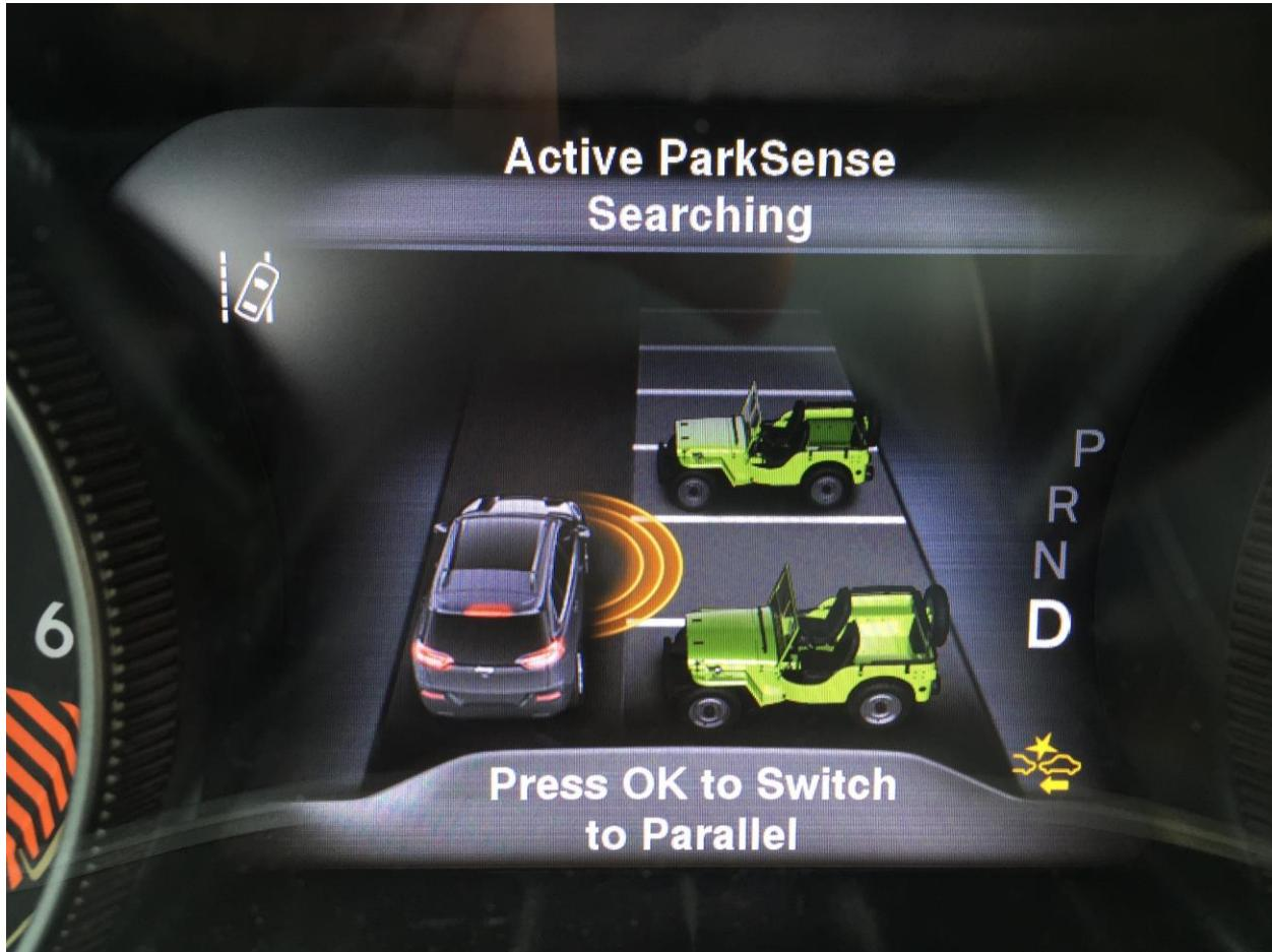
Figure 5: Display while using PAM system
