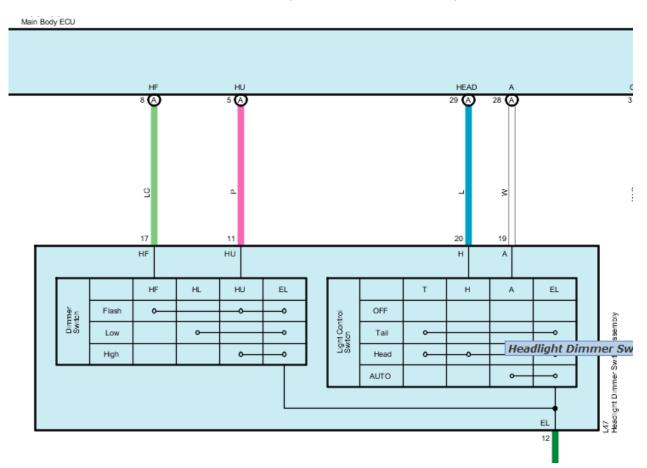
Figure 29. Toyota Prius light switch wiring diagram.
