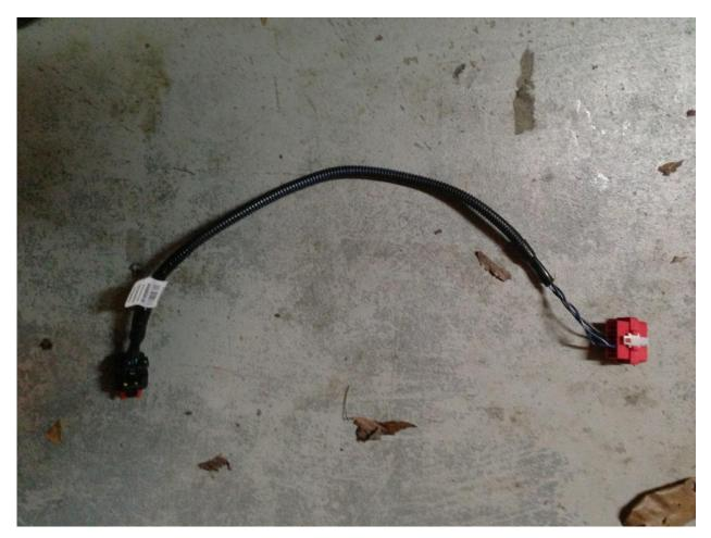
Figure 11: Handmade ECOM-OBD-II connector
