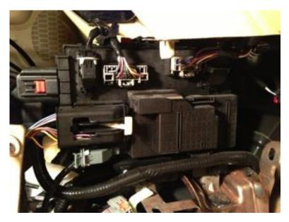
Figure 1: Chassis Computer (SJB) from a 2010 Ford Escape
