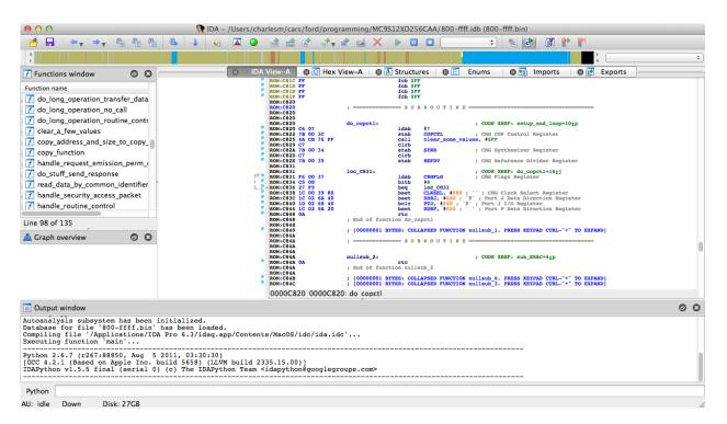
Figure 32. Disassembling the PAM firmware
