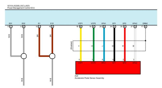
Figure 21. Accelerator Pedal to Power Management Control ECU
