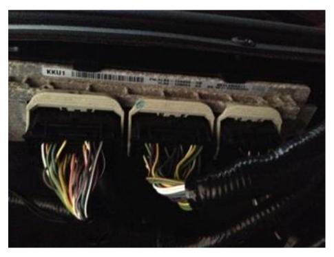
Figure 2: The Powertrain Control Module (PCM) from a 2010 Ford Escape.
