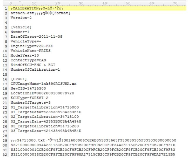
Figure 41. Text view of a Toyota Calibration Update file
