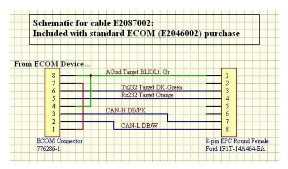
Figure 10. Ecom cable schematic
