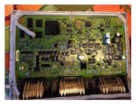
Figure 3: Inside the PCM from Figure 2. The sensors and actuators can be seen to connect to the board on the bottom of the figure.
